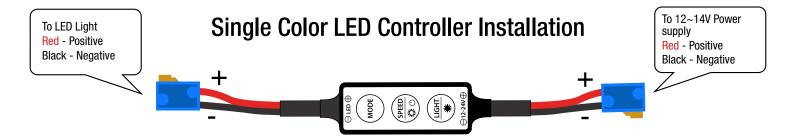
**Installation: 1.** Connect LED strip to LED output on the controller. **2.** Connect power cable to 12~24VDC power supply as shown. Input voltage should match the voltage of the LED strip.
